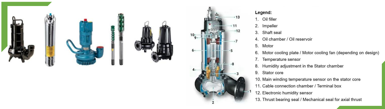
Figure 4. Structure of a submersible pump
